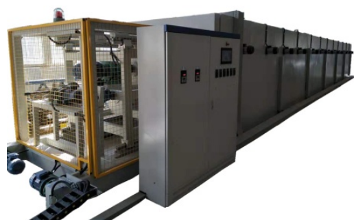
Oven device Different heating zones by adjustable temperature
